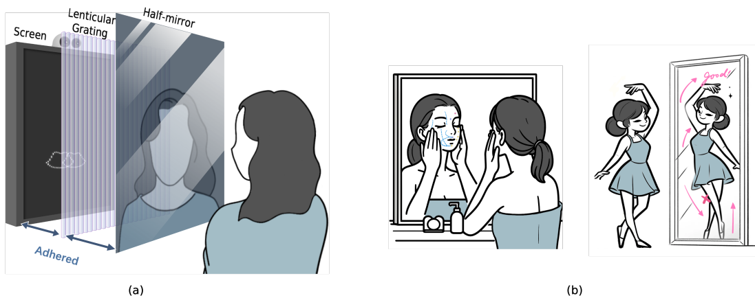
Fig. 1. 3D-Mirrorcle is a smart mirror that overlays augmented reality (AR) with depth perception on a mirror surface. (a) System structure: it employs lenticular gratings between the screen and half-mirror, and adopts depth alignment and segmentation algorithms to project separate images to each eye, merging into a 3D display for an immersive mirror AR experience. (b) Example applications: facial massage and body posture guidance.
